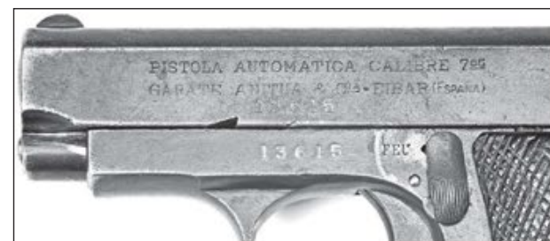
Markings on the Garate, Anita y Cia's slide were in Spanish, but note the "FEU" near the safety lever is the French word for "FIRE."
