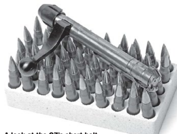
A look at the CZ's short bolt. Note the long claw extractor and dual locking lugs.
