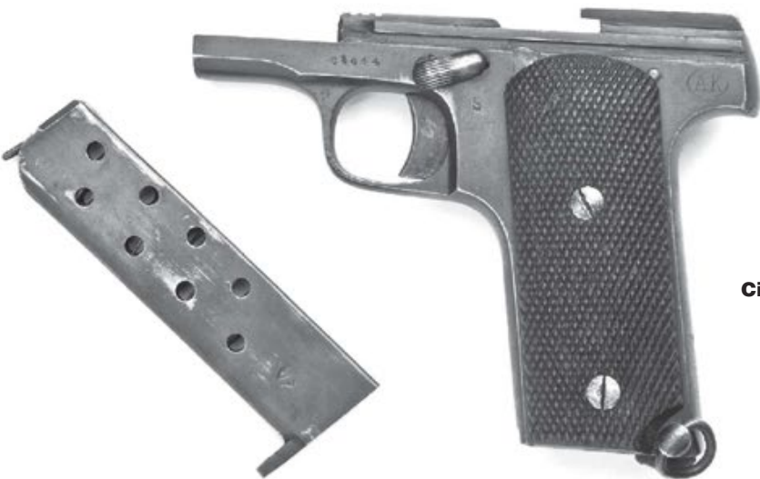
Ruby pistols could be disassembled into five basic components rather quickly. Note the rather massive construction (for a .32 pistol) of the various parts.
